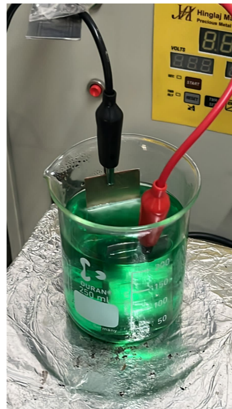
Figure 1: Schematic of the electrodeposition process for NiB nanocrystalline coatings
